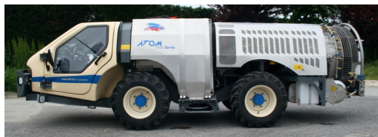
ATOM DISINFECTION can be equipped with a stainless steel AISI 316 tank.
