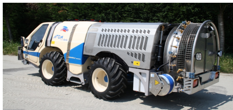
ATOM DISINFECTION can be equipped with a stainless steel AISI 316 tank.
