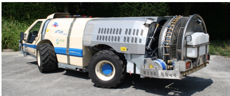
ATOM 1000 DISINFECTION, tank capacity 1000 litres:
