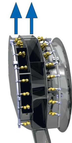
» VAC 896 KIWI blower increases spraying efficacy in all conditions of canopy. Front suction. Double air outlet. Unique guide vanes system designed to evenly reach all parts of canopy. Double nozzle manifolds with different angles produce a cross-spray effect with high coverage efficacy.
