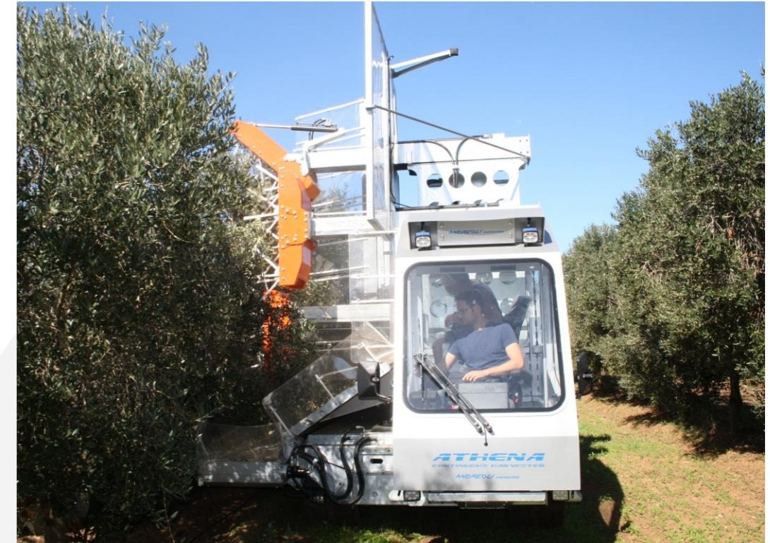
**MACCHINA SEMOVENTE PER LA RACCOLTA DELLE OLIVE
